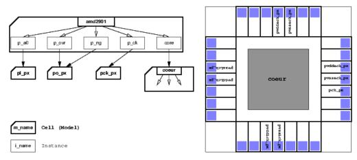
The designer must provide a configuration file that define the rules for the placement of the top-level hierarchy (that is, the pads and the core). This file must be named after the chip's name, by appending \_chip.py (obviously, it is a PYTHON file). For instance if the chip netlist file is called amd2901\_crl.vst, then the configuration file must be named amd2901\_crl\_chip.vst. Example of chip placement configuration file (for AM2901):
