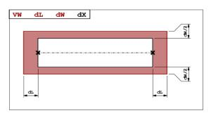
• LCW or RCW for Left/Right Constant Width, create an off-center rectangle of fixed width relatively to the real segment. Note that the SP number is the distance *between the edge* of the real segment and the edge of the generated real rectangle (*not* from the axis). It is often zero.
