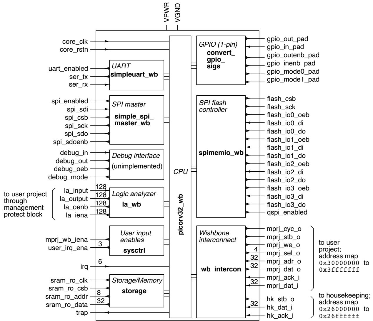
All signals connect to the housekeeping subsystem unless otherwise specified.
