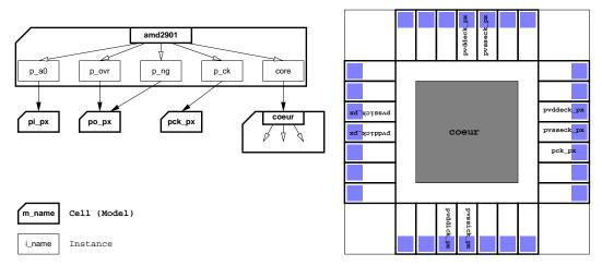
The designer must provide a configuration file that define the rules for the placement of the top-level hierarchy (that is, the pads and the core). This file must be named after the chip's name, by appending <code>\_chip.py</code> (obviously, it is a PYTHON file). For instance if the chip netlist file is called <code>amd2901\_crl.vst</code>, then the configuration file must be named <code>amd2901\_crl\_chip.vst</code>. Example of chip placement configuration file (for <code>AM2901</code>):
