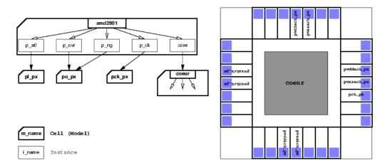
The designer must provide a configuration file that define the rules for the placement of the top-level hierarchy (that is, the pads and the core). This file must be named after the chip's name, by appending <code>\_chip.py</code> (obviously, it is a PYTHON file). For instance if the chip netlist file is called <code>amd2901\_crl.vst</code>, then the configuration file must be named <code>amd2901\_crl\_chip.vst</code>. Example of chip placement configuration file (for <code>AM2901</code>):
