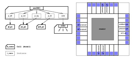
The designer must provide a configuration file that define the rules for the placement of the top-level hierarchy (that is, the pads and the core). This file must be named after the chip's name, by appending \_chip.py (obviously, it is a PYTHON file). For instance if the chip netlist file is called amd2901\_crl.vst, then the configuration file must be named amd2901\_crl\_chip.vst. Example of chip placement configuration file (for AM2901):
